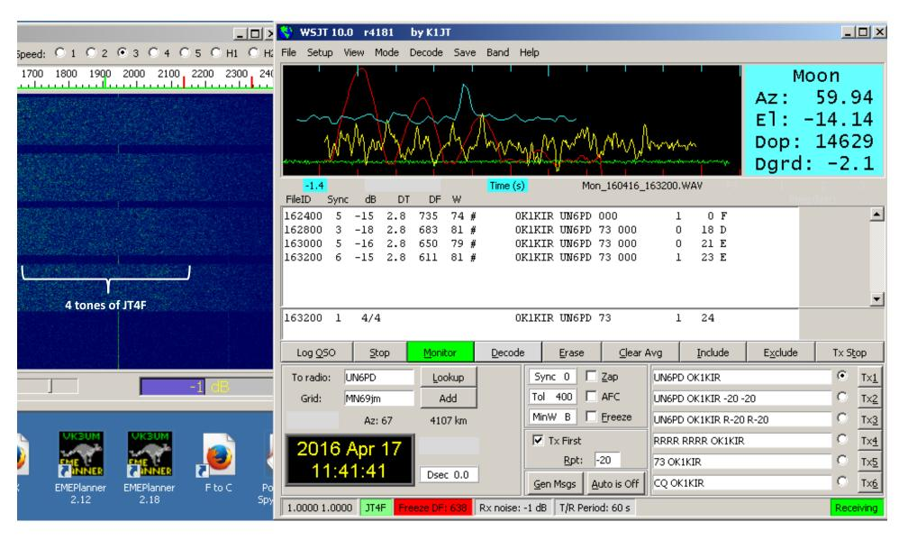
16.4.2016 3cm EME QSO OK1KIR–UN6PD Audio files 1624 till1632 shows the UN6PD signal with high spreading (prediction ≈188 Hz) received at OK1KIR (files were post-processed after QSO was finished). Picture shows WSJT capability to decode such very weak JT4F signal (almost unvisible traces) with default settings and even with MinW=B instead of more suitable E or D (for such high spreading).
