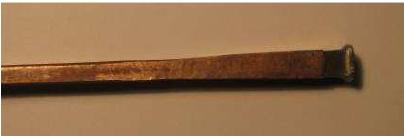
Fig.1 Semi-finished copper horn from Cu WG R220 (WR42) with horn steel gusset when hammered in
