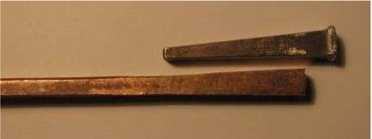
Fig.2 Semi-finished copper horn from Cu WG R220 (WR42) with horn steel gusset excluded outside
