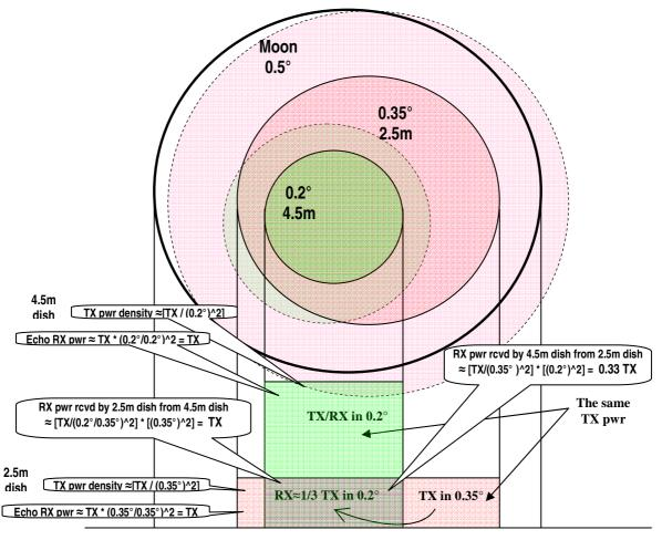
The best case: Bigger dish(4.5m) receives 1/3 of TX power transmitted by smaller dish(2.2m) In opposite way, the smaller dish receives the full transmitted power<sup>1</sup> from bigger dish!
